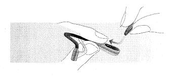
d) Refit the battery. Ensure that the side with the+ sign faces upwards.
