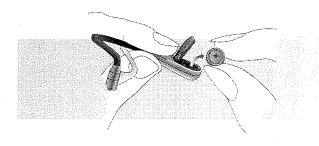
b) Lift up the battery compartment cover at a right angle and pull it away in the direction of the battery compartment.
