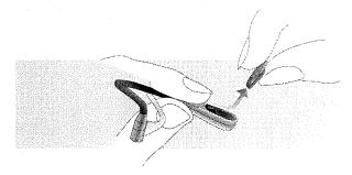
c) Hold the screw-locking battery compartment cover at a right angle and slide it in from the side of the battery compartment.
